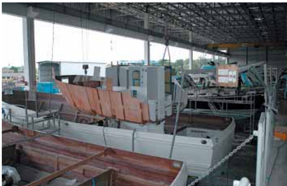
Top: Modular construction, with components assembled on the factory floor, speeds construction. This module contains the forward staterooms and heads for the 44 Europa.
